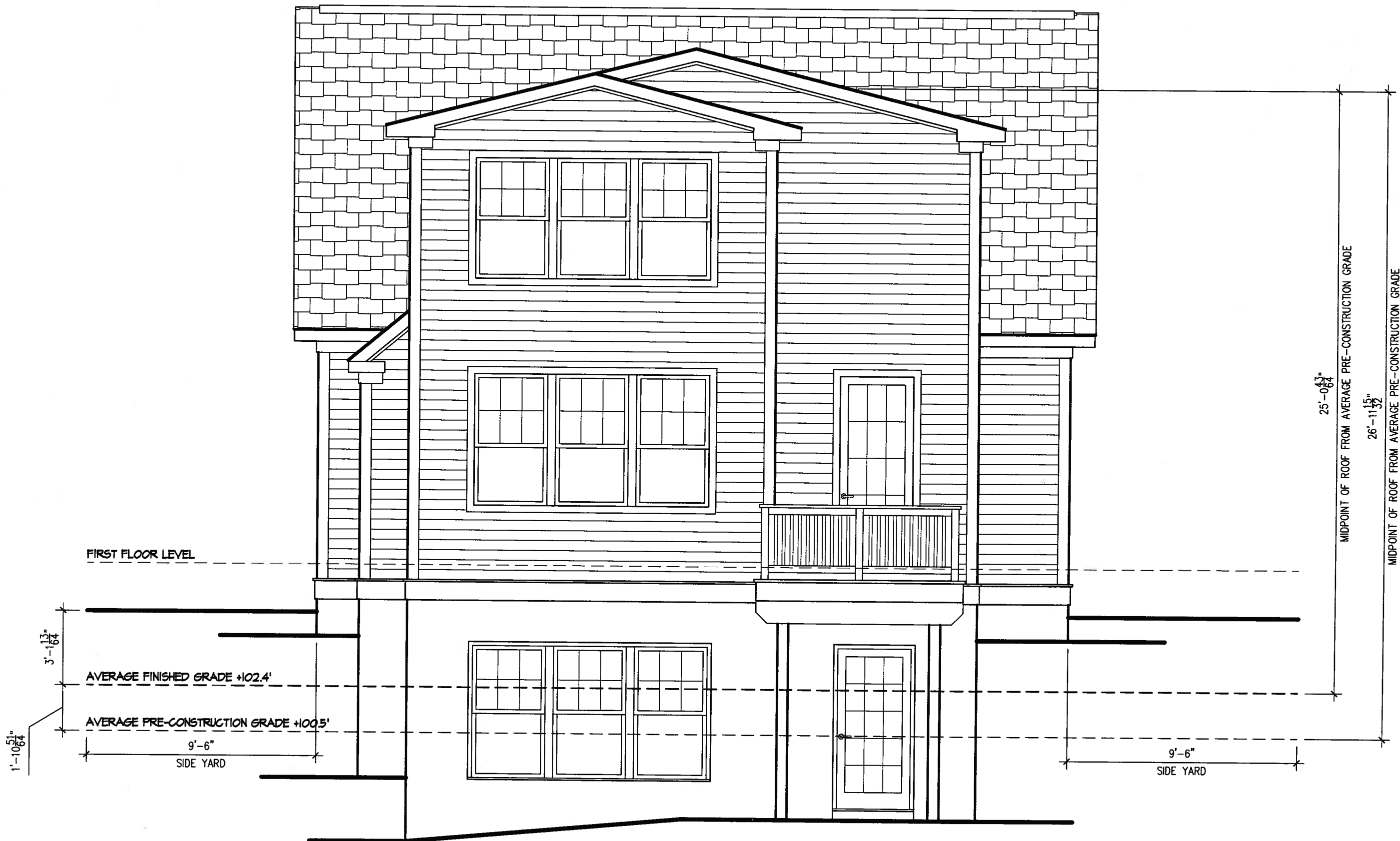
1 PROPOSED REAR ELEVATION A6 SCALE: 1/4" = 1'-0"
