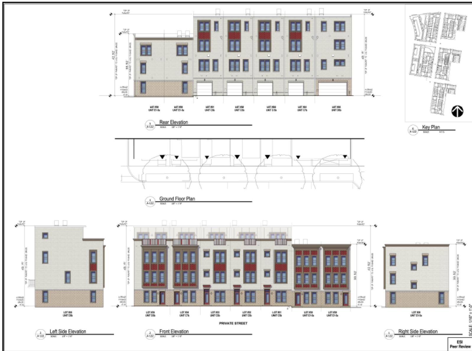
Figure 9. Alley dwelling elevations (northern strip).
