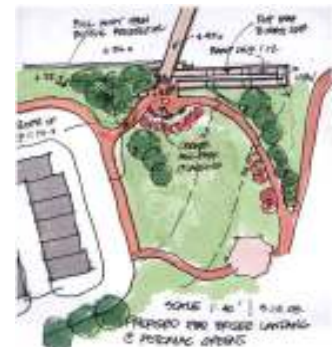
Figure 9: Staff Recommended Ped. Bridge Landing
