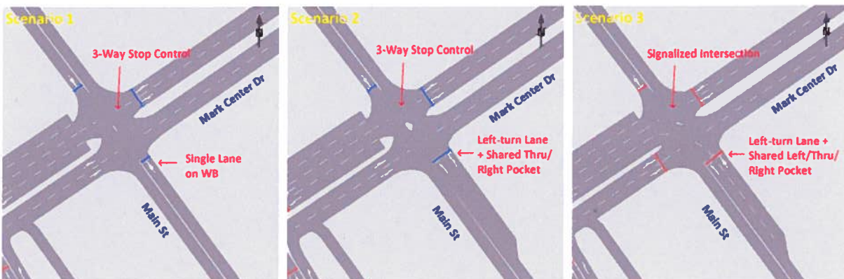
Figure 5: Lane Configuration and Traffic Control Device Alternatives at the Main Street and Mark Center Drive Intersection
