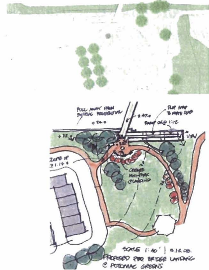
Figure 9: Staff Recommended Ped. Bridge Landing
