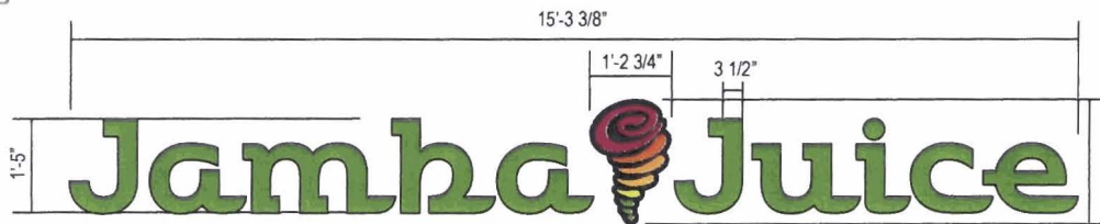
A Channel Letters Front View Scale - 1/2" = 1'-0"
