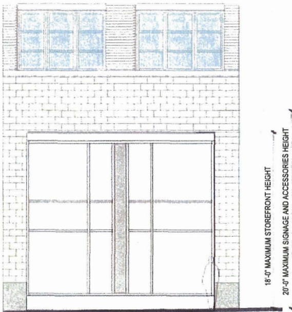
Storefront system for center demising wall option Double and single side door options can also be integrated.
