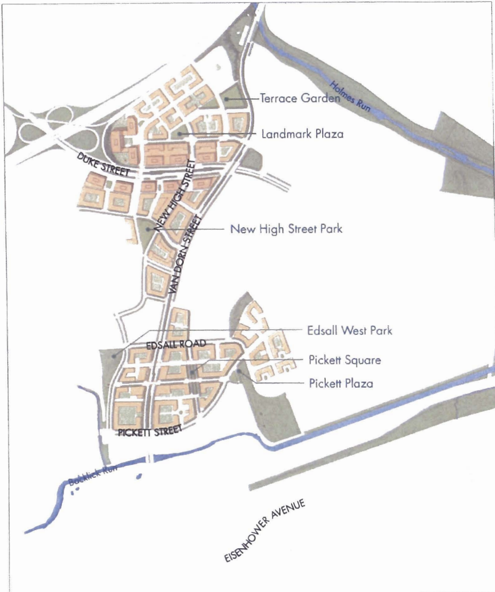
Figure 6-13. Open Space Plan. A number of small urban parks will provide nearby open space for new mixed-use developments. All areas within new mixed-use developments are within an easy walk of one of these public open spaces.
