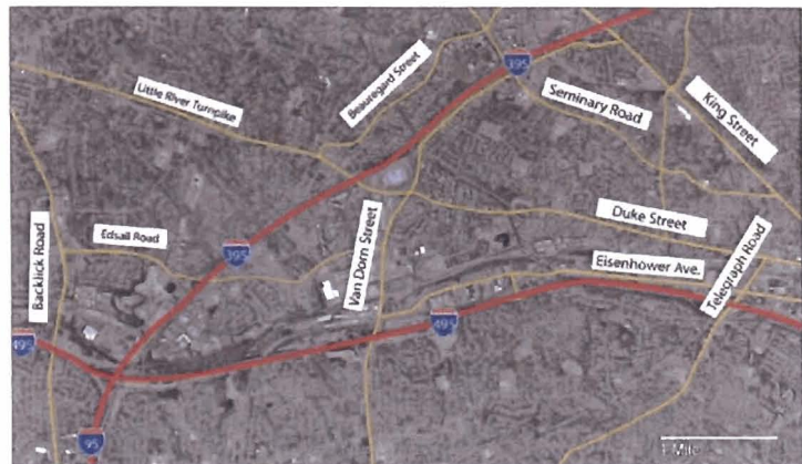
Figure 5-2. This figure illustrates the limitations of the local arterial roadway and expressway system in handling north-south traffic. Van Dorn Street is the only north-south link across the Capital Beltway between Telegraph Road and Backlick Road, a distance of six miles. Its location makes it a desirable short-cut for I-395 traffic to and from southeastern Fairfax County or across the Woodrow Wilson Bridge
