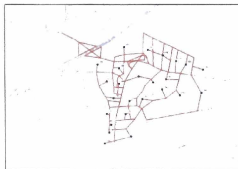
Figure 5-18. The planning area was divided into a number of subzones, and additional links were added to the street system for analysis of future conditions.
