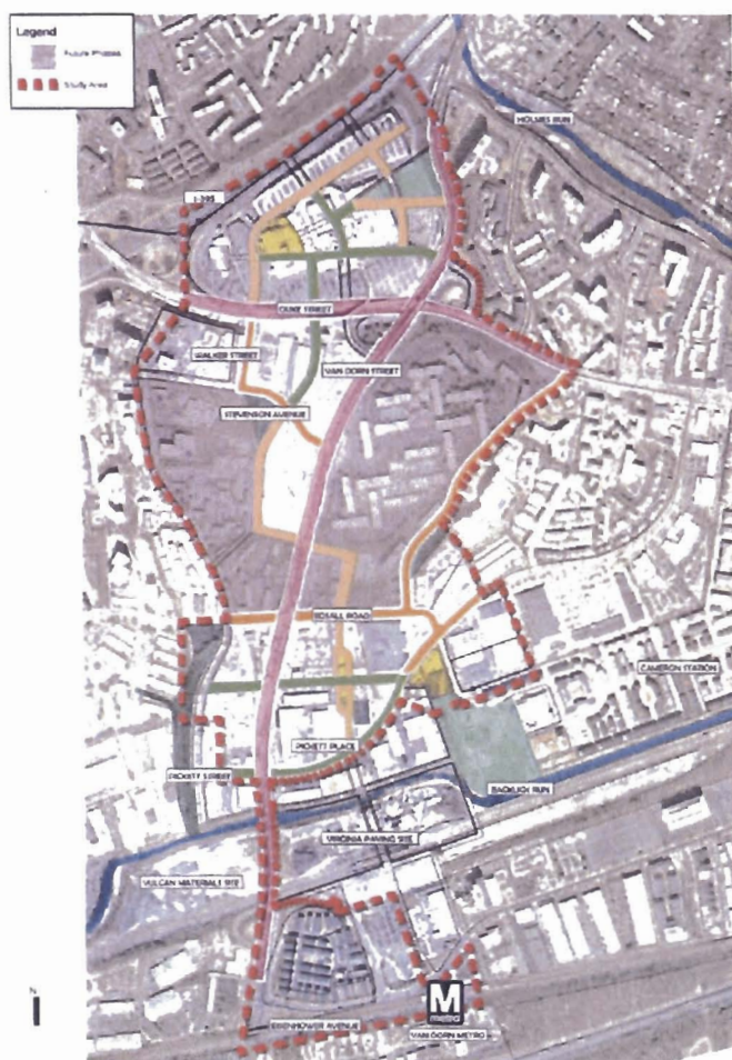
Figure 9-1 Stormwater Management Strategies. This figure illustrates the application of strategies outlined in Table 9-4 on the following page. Color codes in the table show application of appropriate strategies to streets and open spaces.
