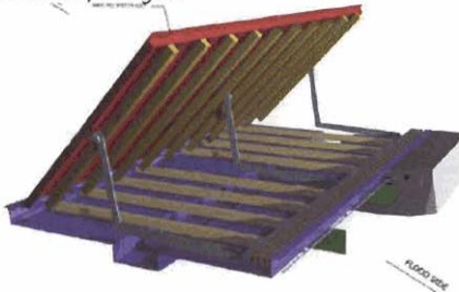
Ballasted flood gate
