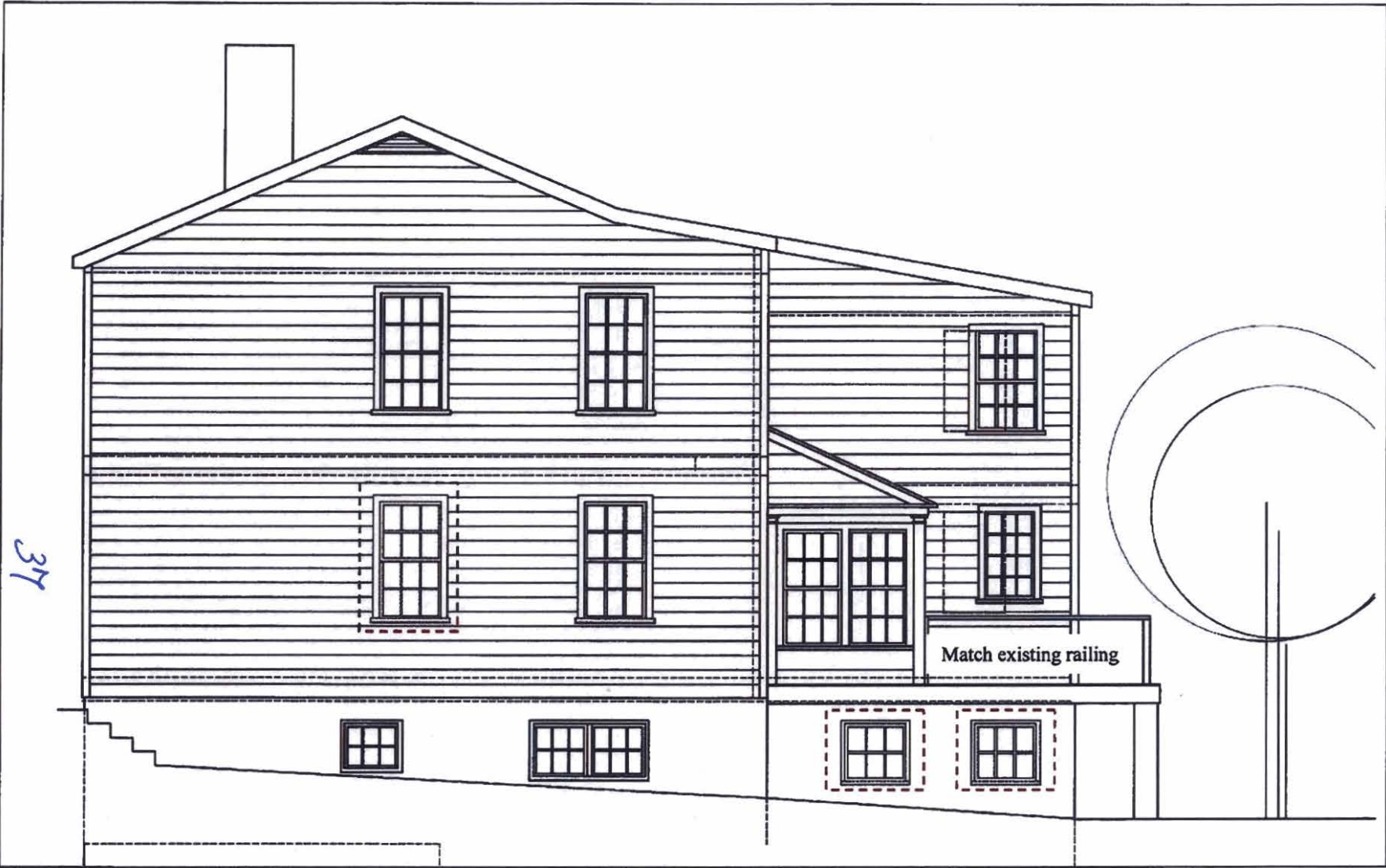
Figure 11: Proposed south (side) elevation with proposed new windows shown surrounded by dashed red lines.
