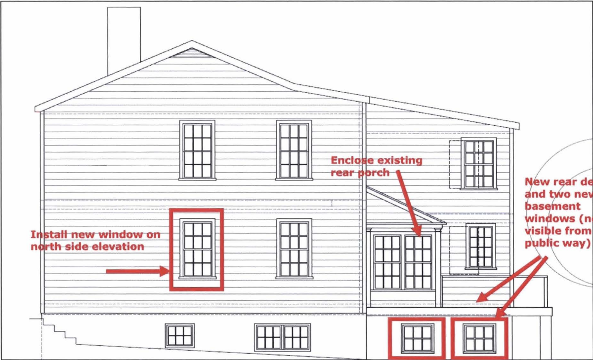
Figure 10: Proposed south (side) elevation with proposed new windows shown surrounded by red lines.
