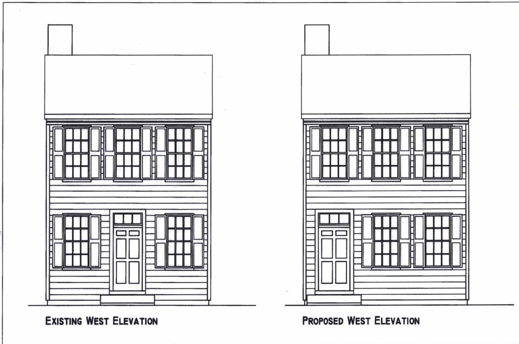
Figure 7: Existing and proposed west (front) elevation.
