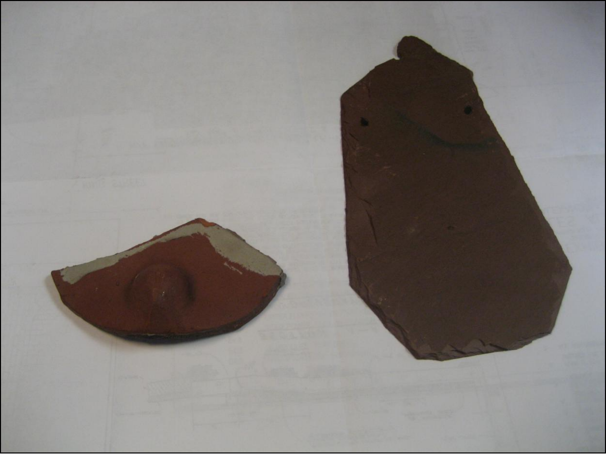
Figure 3. Piece of existing clay tile with decorative knob (left) and sample of red slate (right).
