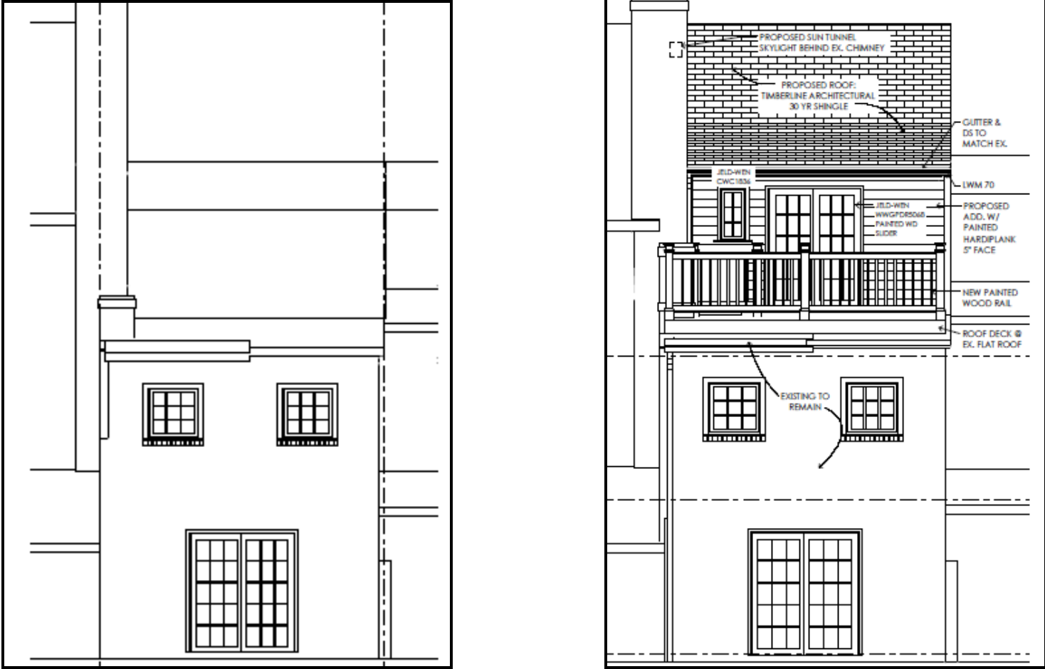
Figure 6: Existing and Proposed Rear Elevations
