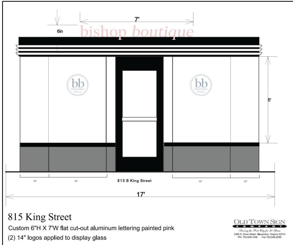
Figure 2: Drawing showing proposed signage. Note that the window decals will be white, not blue.
