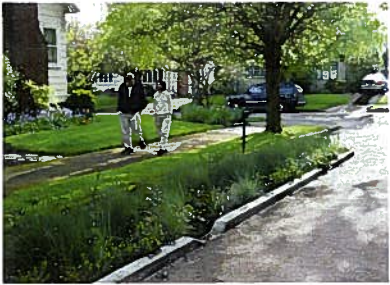
Street tree in planting areas that integrate stormwater management
