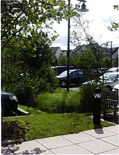
Example of a bioretention planting strip in a parking lot
