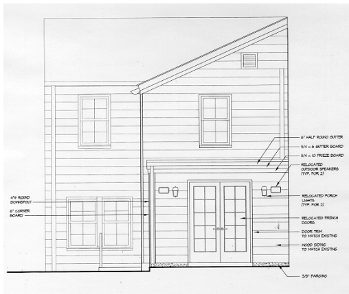
Figure 1 Rear elevation proposed addition
