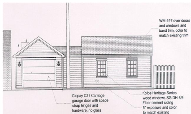
**Figure 2** Proposed alley elevation
