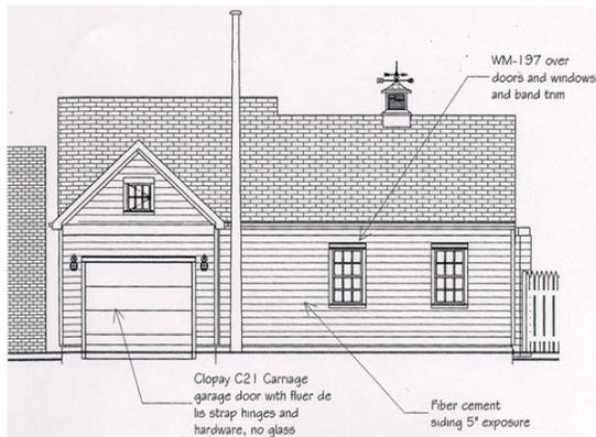
**Figure 1** Previous alley elevation
