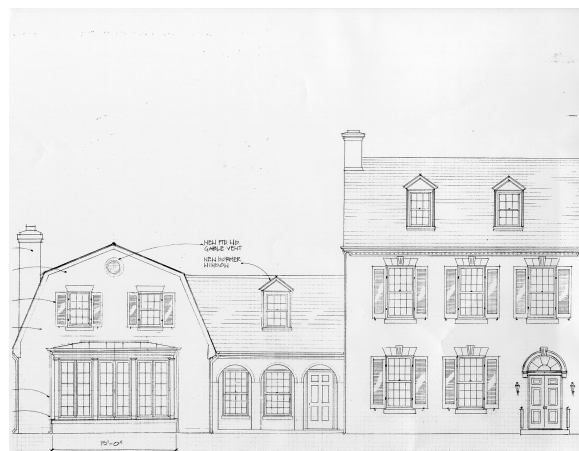
Figure 1 - Proposed alterations to front elevation of addition
