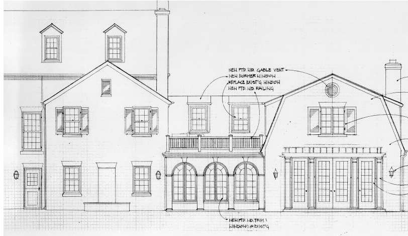
Figure 3 - Rear elevation showing proposed elevations to addition
