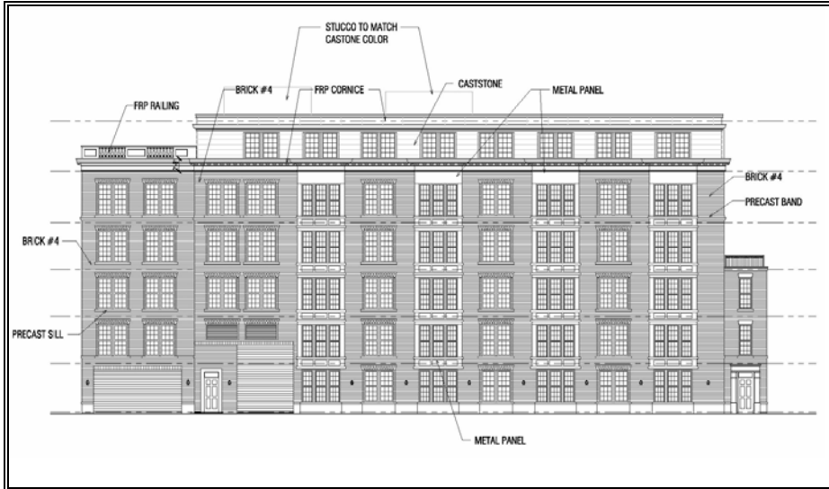
Figure 2 - Previously approved South elevation, 01/18/2006
