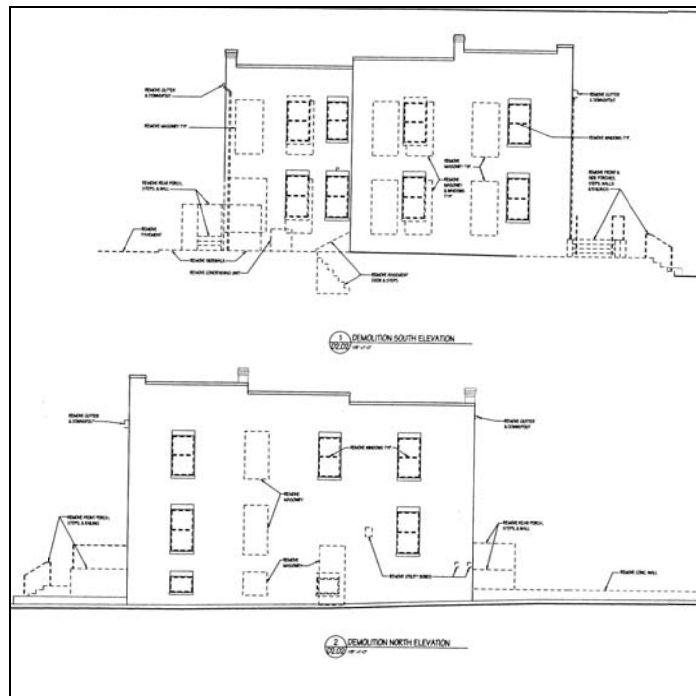
Figure 4. Proposed demolition for south and north elevations.
