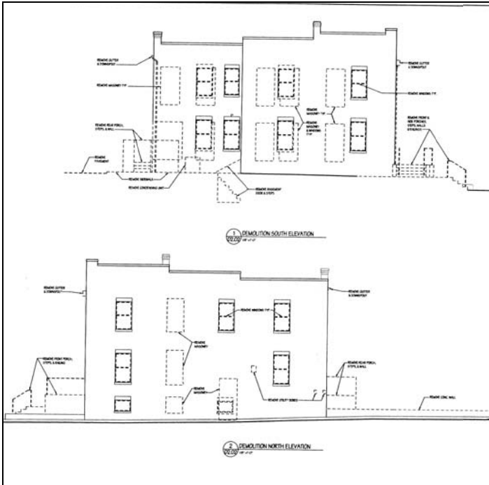
Figure 4. Proposed demolition for south and north elevations.
