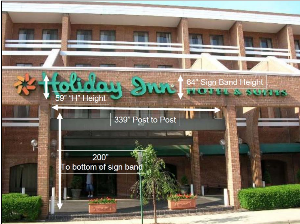
Figure 4. Existing wall sign with measurements.
