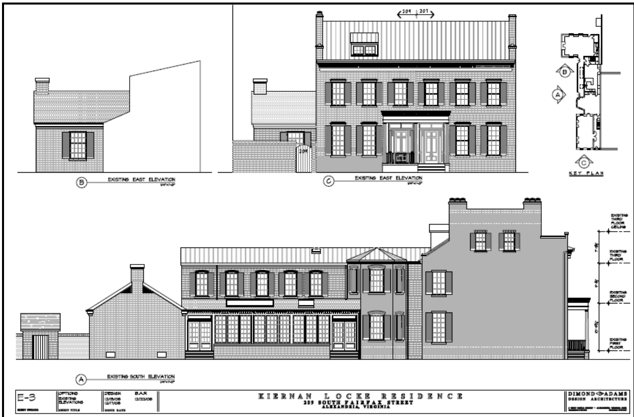
Figure 9: Existing East and South Elevations
