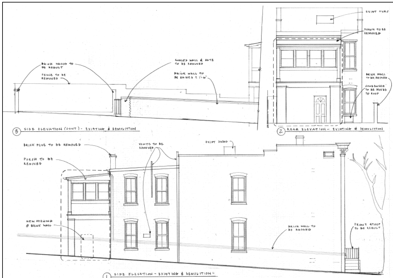
Figure 7. Proposed demolition in elevation.
