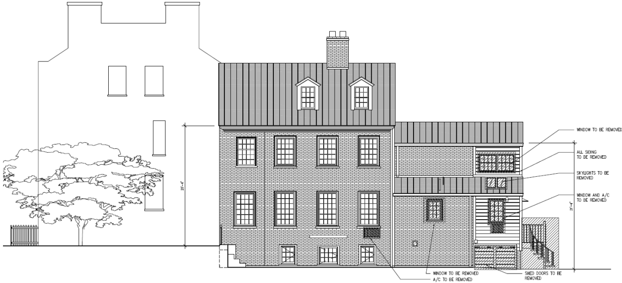
EXISTING SOUTH ELEVATION
