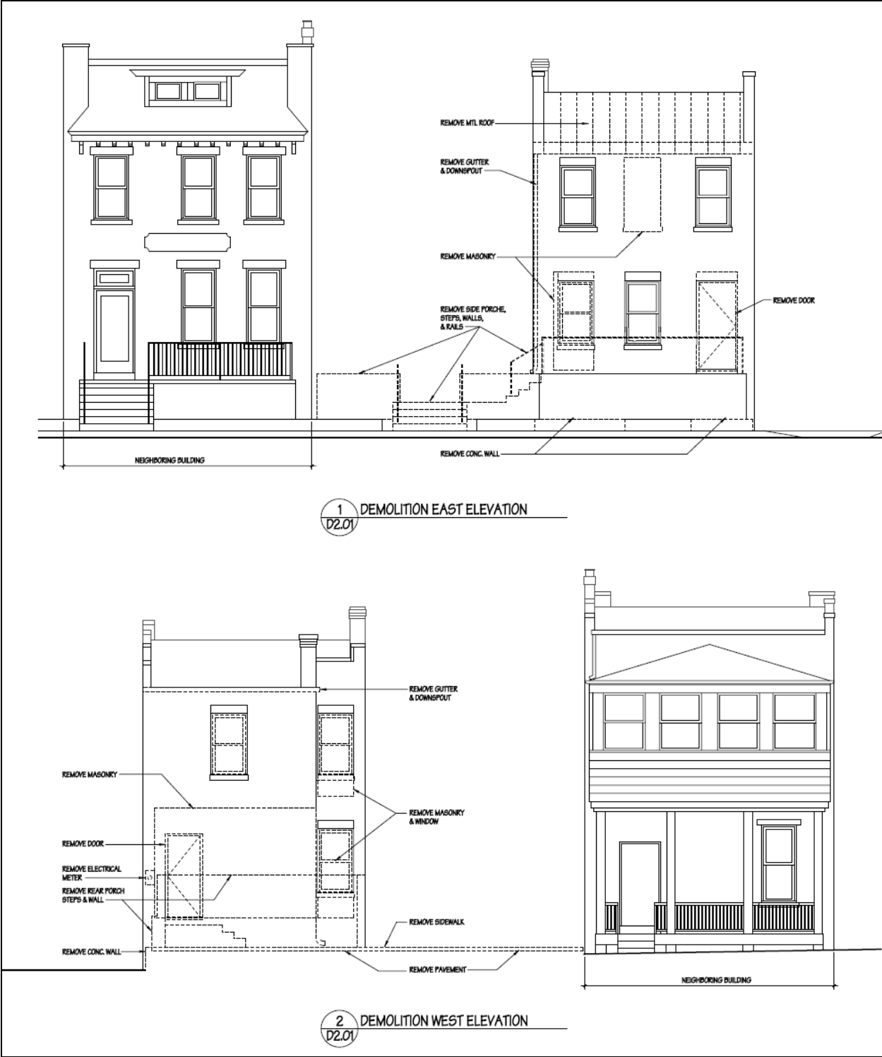
Figure 9. Areas of approved demolition/encapsulation on east and west elevations.
