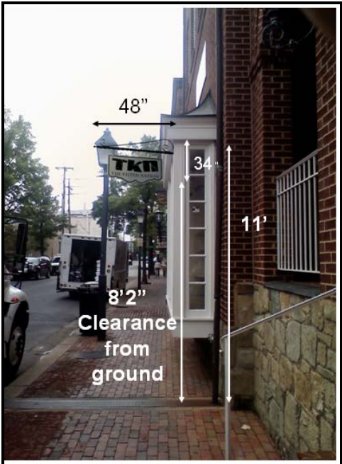
Figure 4: Proposed clearances for hanging sign.
