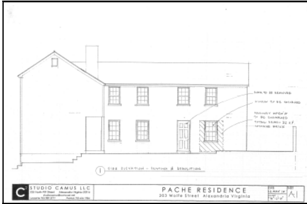
Figure 2: Existing east elevation with area of demolition/alterations.
