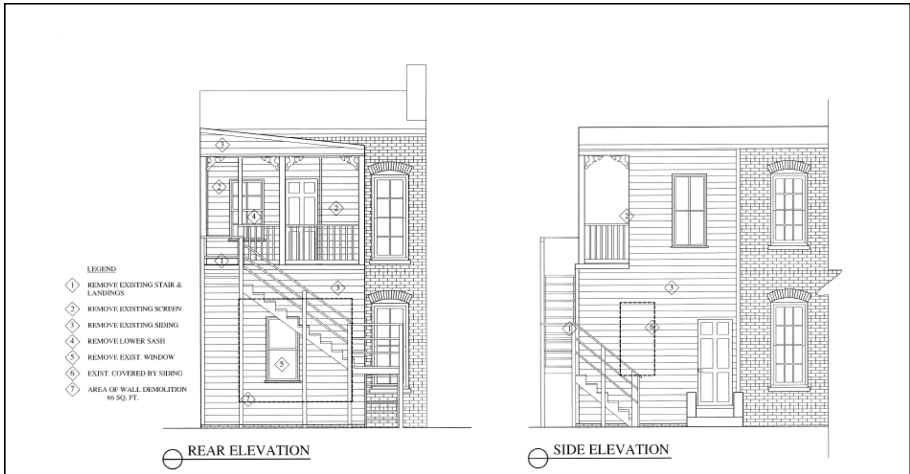
Figure 3: Existing rear (south) and side (east) elevations of the ell outlining proposed areas of demolition
