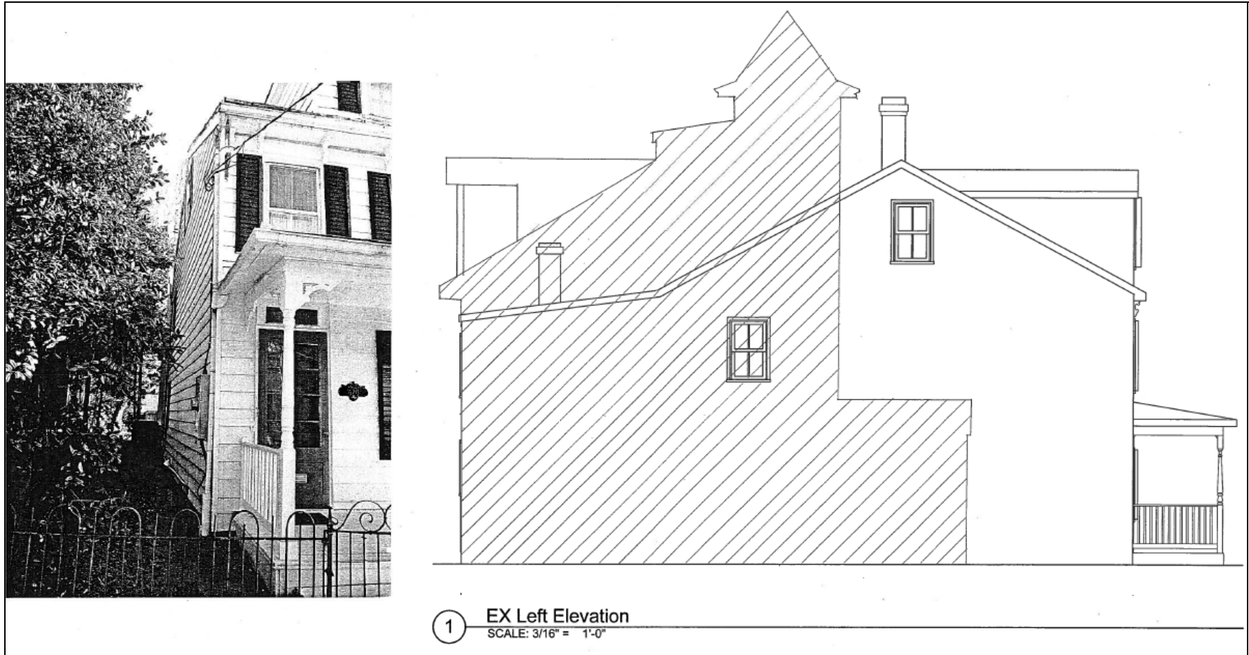
Figure 9. Existing side (north) elevation, showing massing of proposed addition and areas of demolition/encapsulation.
