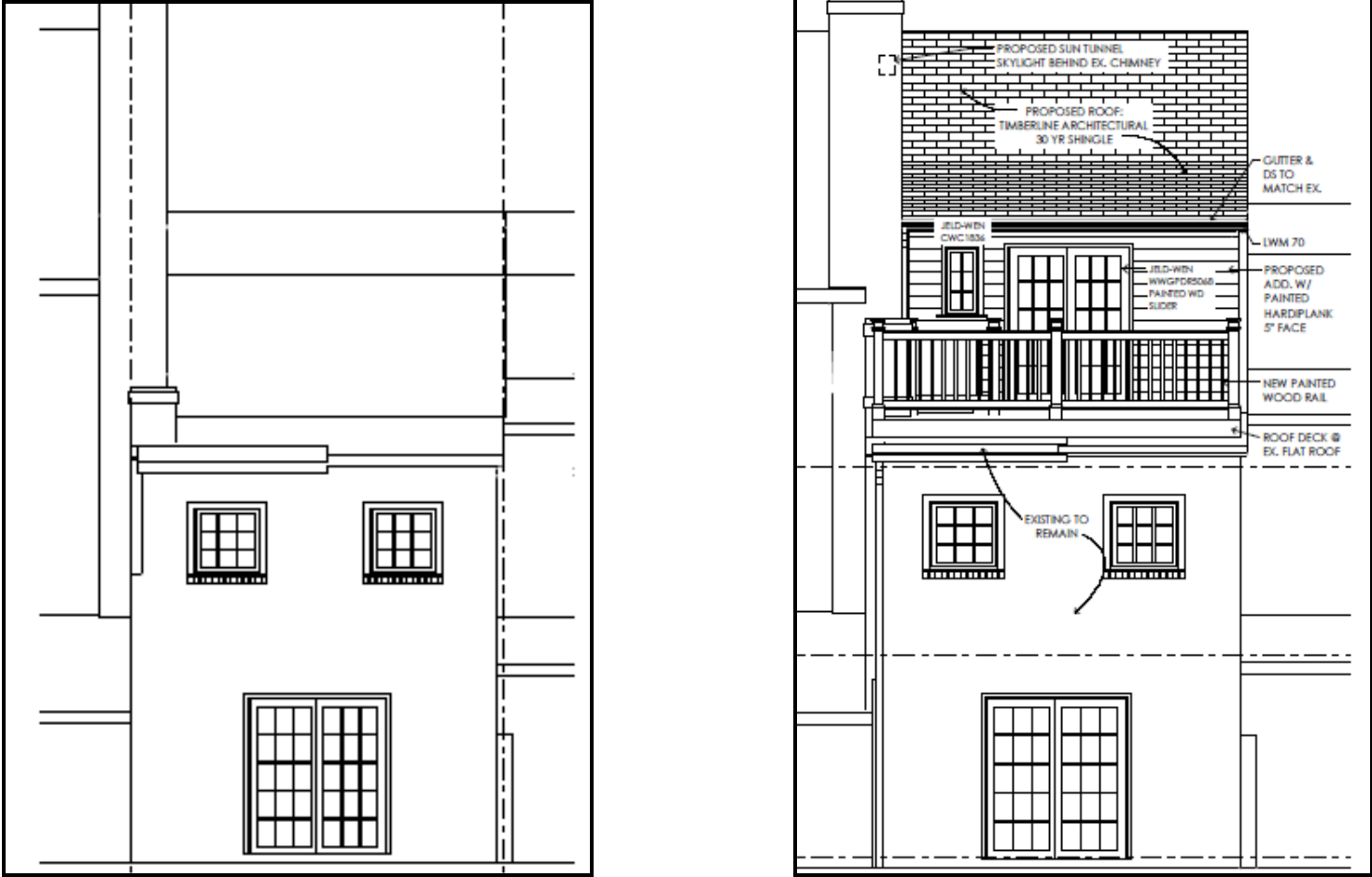
Figure 6: Existing and Proposed Rear Elevations
