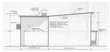
Figure 2 - North elevation
