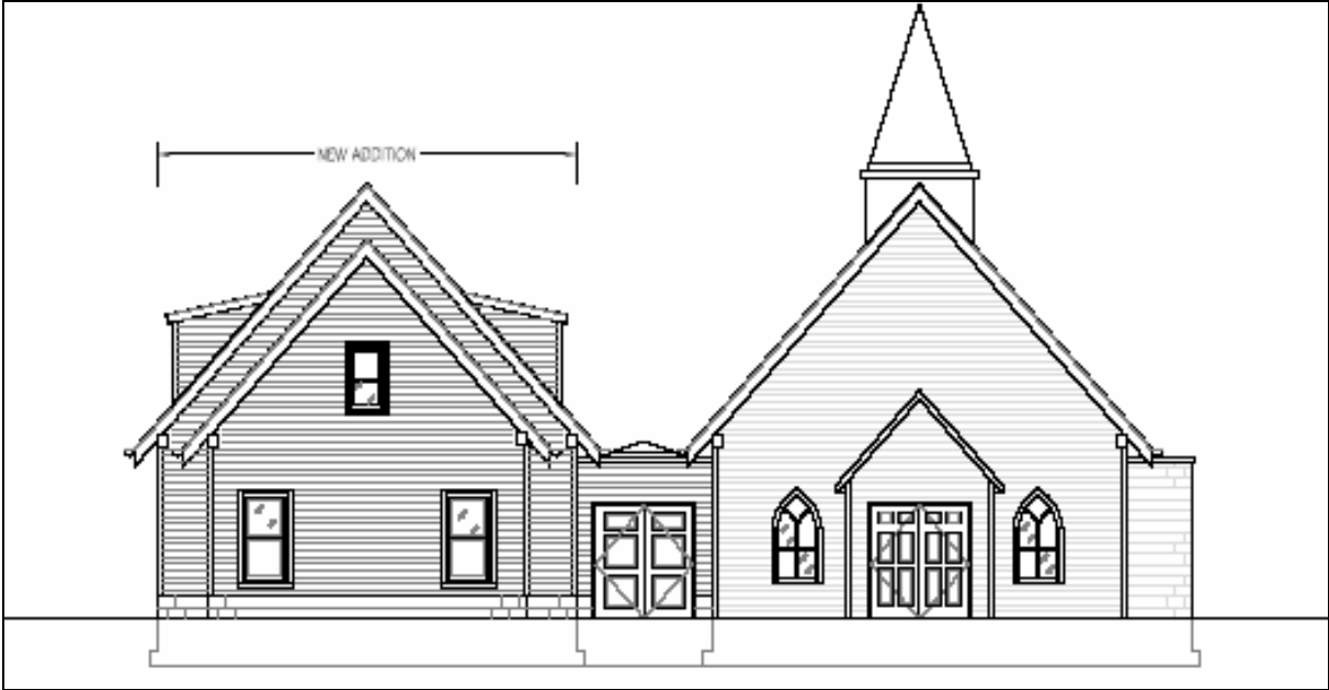
Figure 4: Front elevation showing proposed addition
