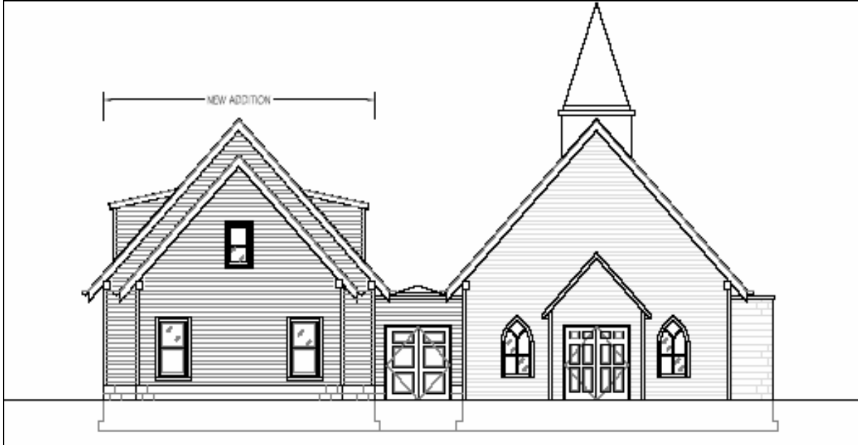
Figure 4: Front elevation showing proposed addition
