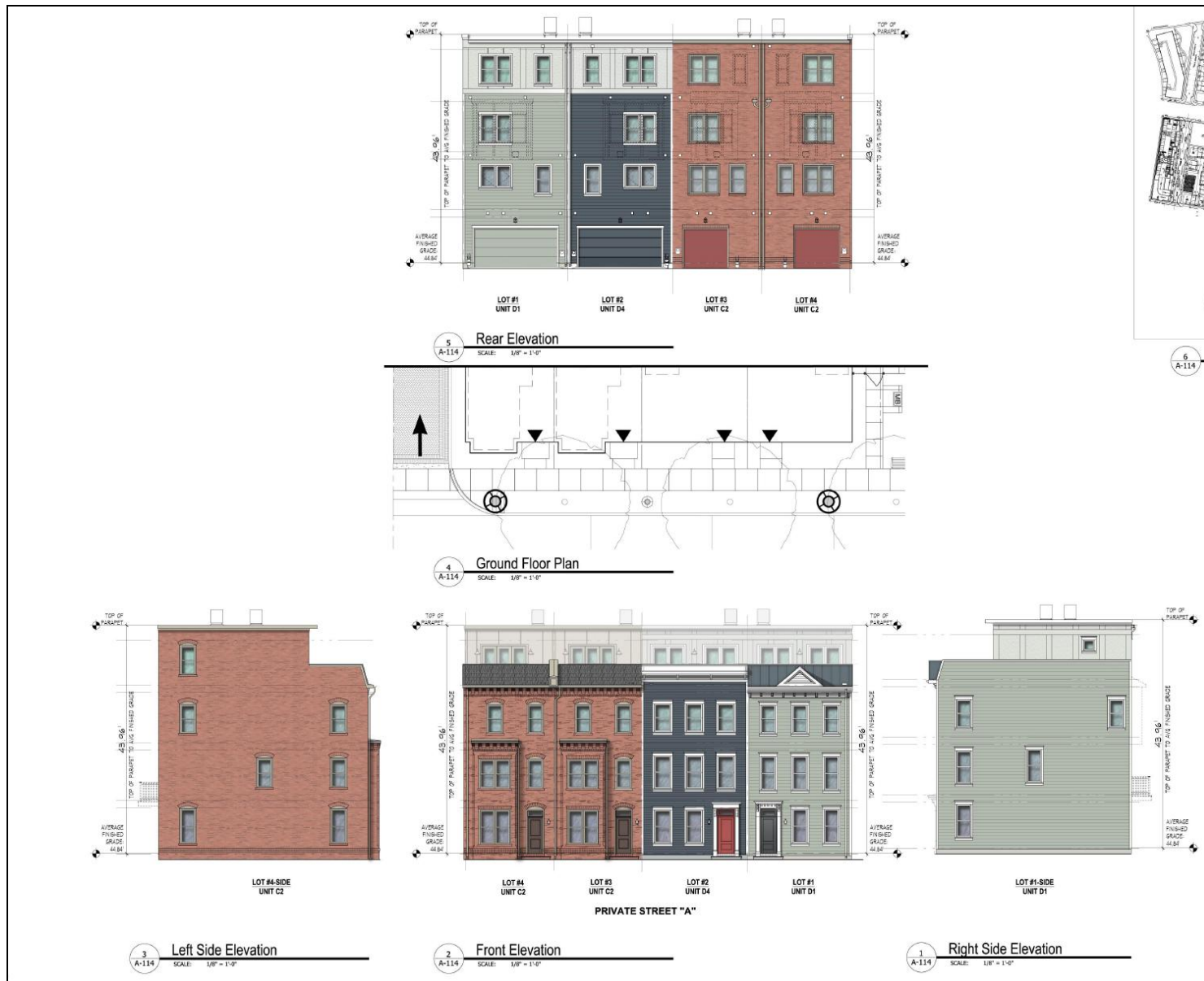
Figure 6. Private street, southernmost townhouses, strip elevation.
