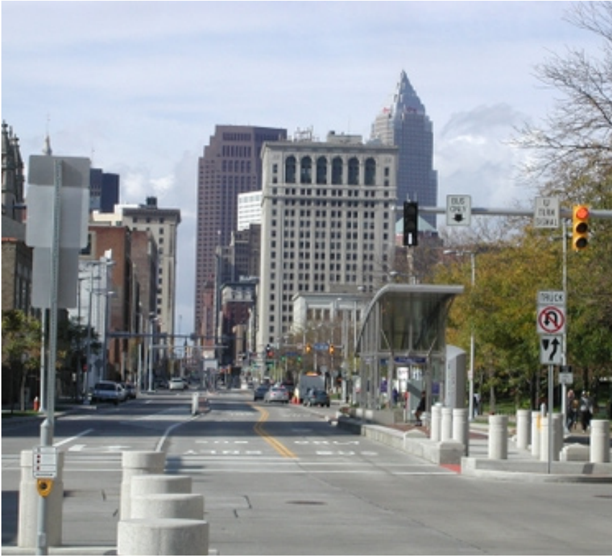
Far side (of the intersection) bus stop in Cleveland along the Healthline BRT
