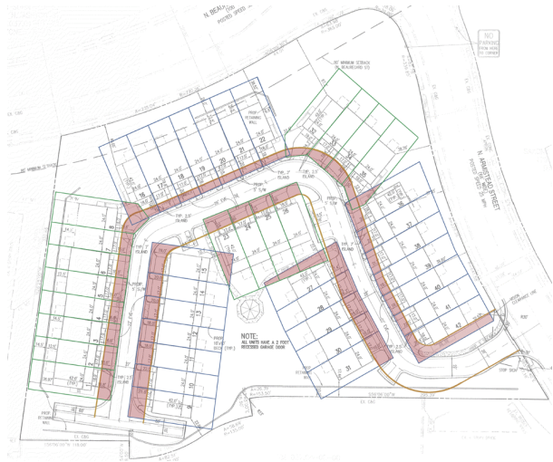
Applicant's Proposal w/ Townhouse Lot Lines. Shaded areas depict overlapping lot lines &/or ROW.
