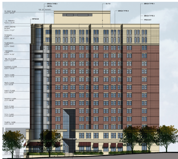
East Elevation on Andrews Lane
