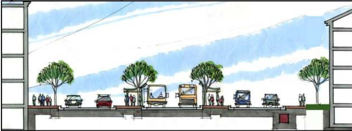
Figure 2. Two-Lane Transitway Located in Median
