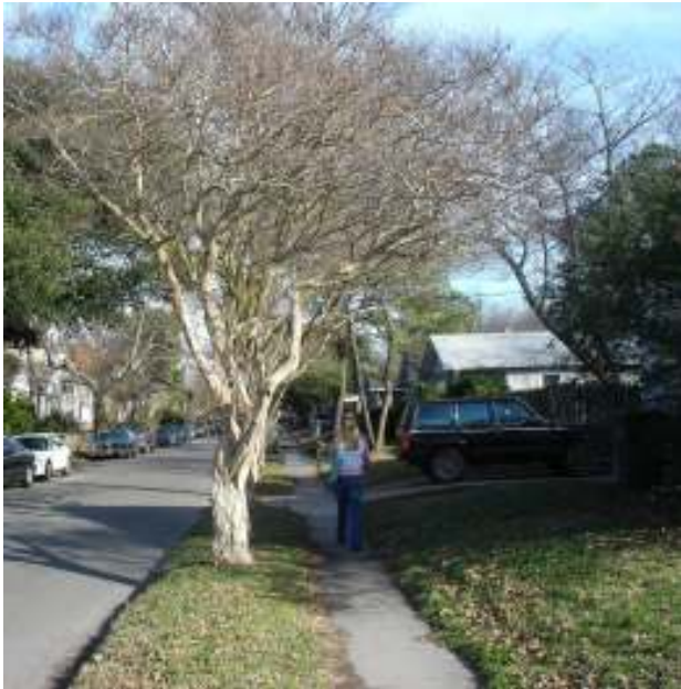
Planting strips accommodate a variety of vegetation that help separate pedestrians from traffic, define the character of the overall street, enhance adjacent buildings and open space, and allow natural stormwater infiltration.
