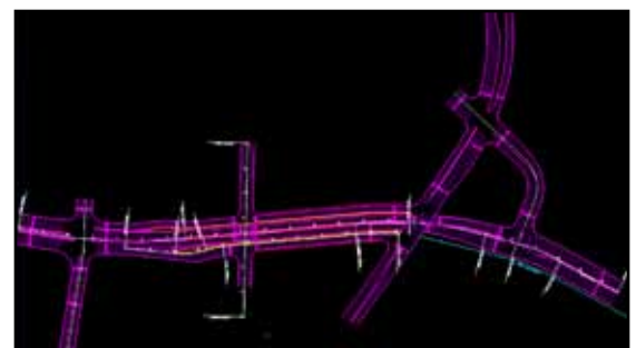
Figure 5-11. Frontage roads alternative. Alignment of Duke Street and New High Street with frontage roads along Duke Street at plaza level and through traffic operating at a lower level at the existing grade of Duke Street.
